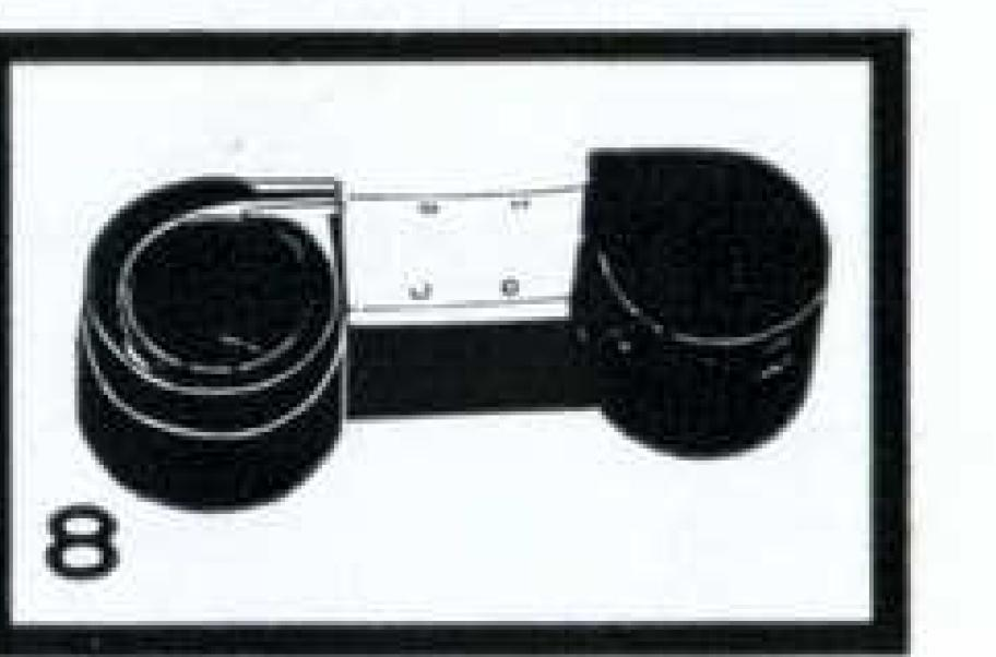
Fit the remaining cap over the larger chamber and secure it with cellotape. The film should be strictly parallel.
