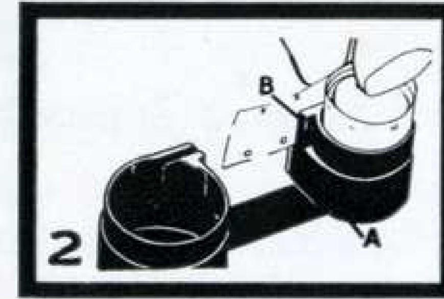
Place the rolled film in the smaller chamber of the cassette.
