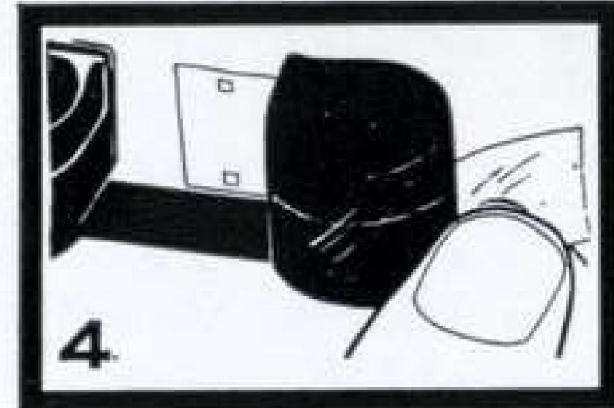
Secure cover with a piece of cellotape so the cover is tight.
