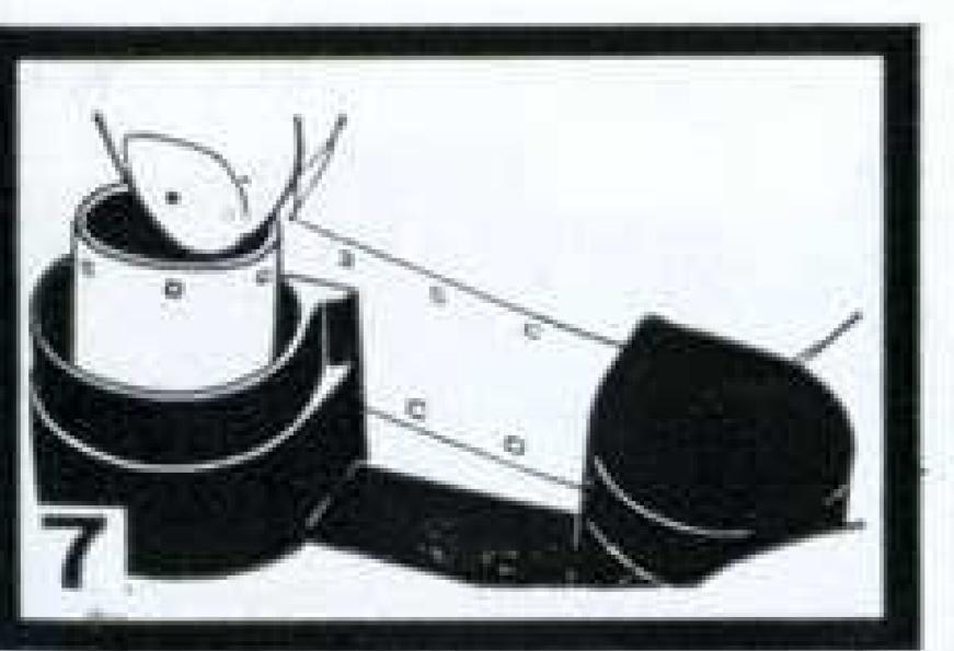
Wind 1½ times around the drum so that the film may become parallel to the drum side. Place the film into the magazine.
